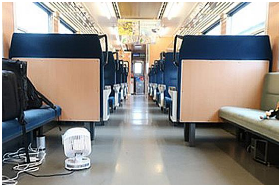
Figure 9. Main test train carriage setting showing more discrete location of odor diffuser and fan
